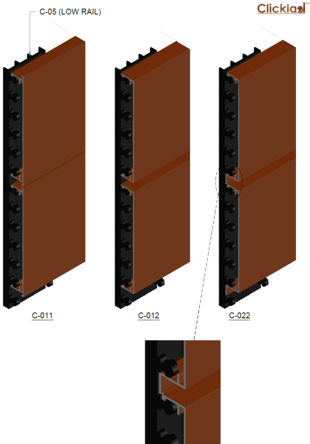
9.3.1 Figure of the Click Rail and Clickclad Interaction. C-011 demonstrates Clickclad Tight gap system, C-012 demonstrates Clickclad open gap system and C-022 demonstrates Clickclad waterproof system.
